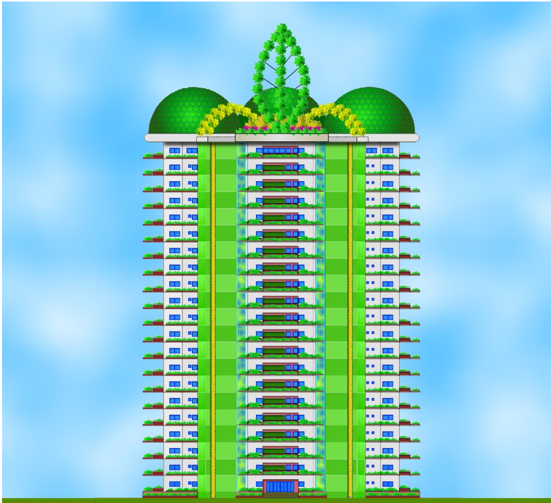
Figure 5. Front view of the building with the biomimetic roof. The three domical forms and the hydrophilic bumps are seen. Source: Author's design portfolio
